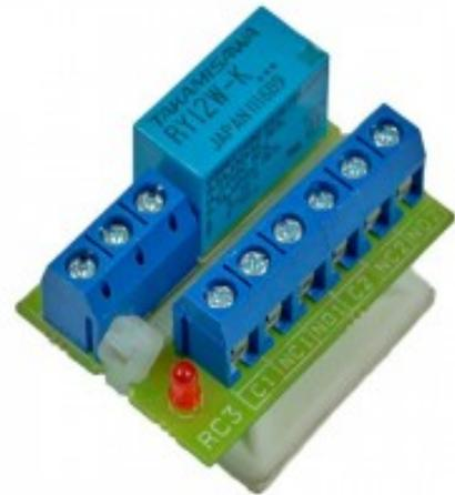
The RC 3 is a very compact and universal relay card with dual alternating (NC / NO) relay function. Connection is provided via screw terminal with wire protection.
